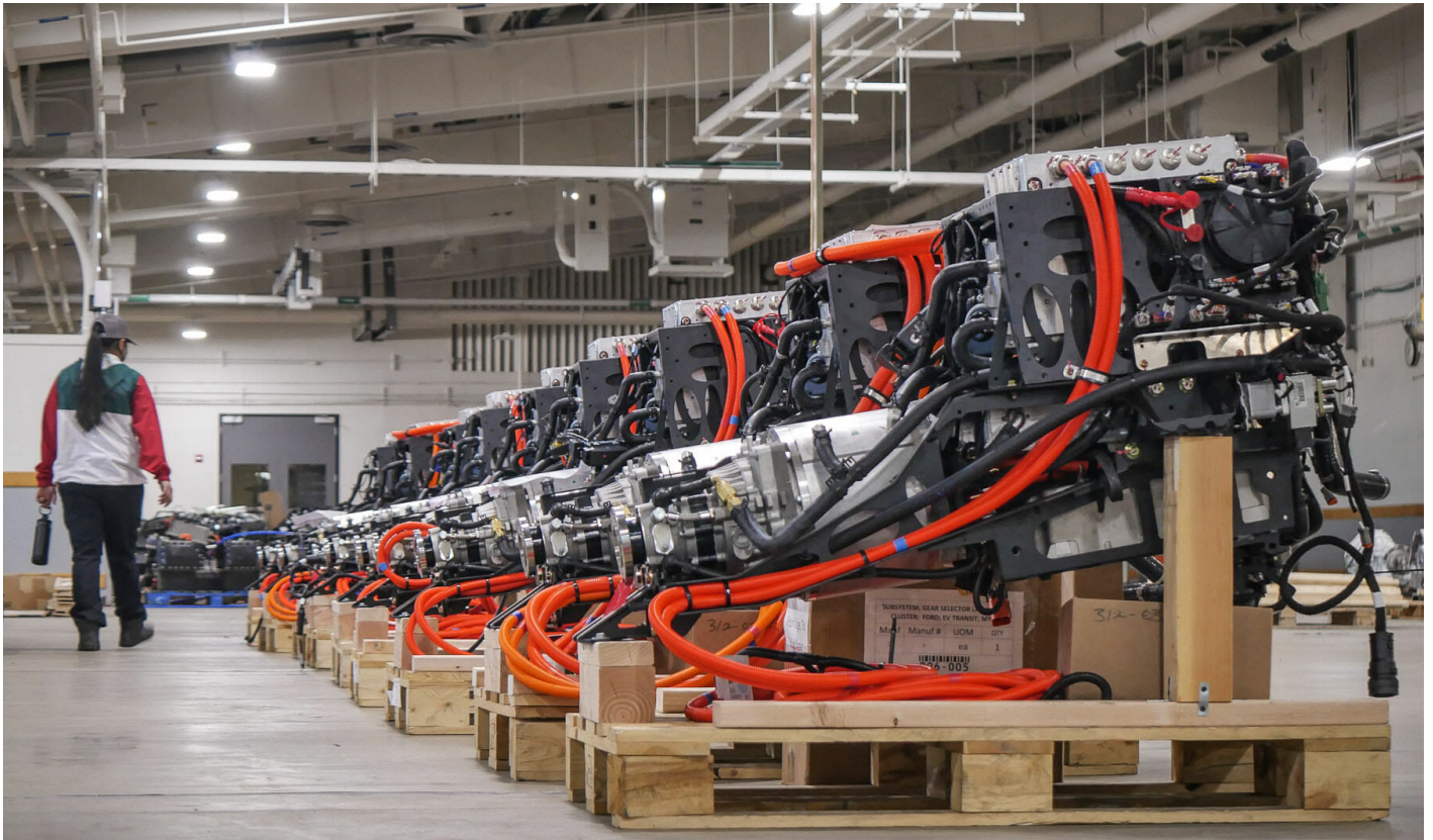
Assembled electric powertrains ready for installation into Lightning Electric Transit 350HD vehicles
