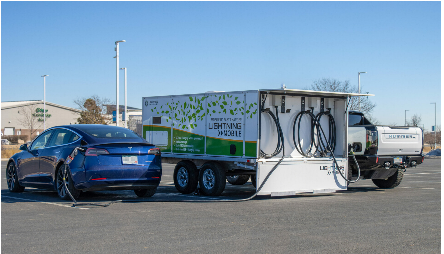
Lightning Mobile provides on-location EV charging that is applicable to situations commonly found at airports, such as Dallas Fort Worth International. (Photo: Lightning eMotors)
