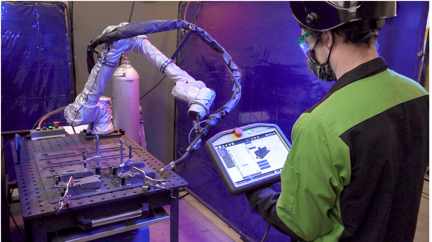
Manufacturing Engineer Austin Laurel programs a collaborative welding robot for automated production of volume parts. (Photo: Lightning eMotors)
